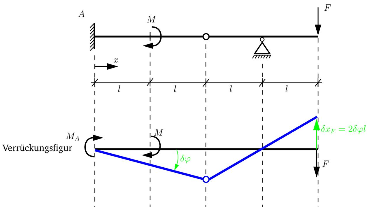
$$\delta W = M_A \delta \varphi - M \delta \varphi + F \delta x_F = \delta \varphi (M_A - M + F \cdot 2l)$$
